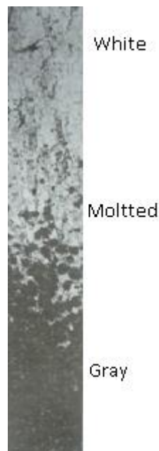
Fig.7.7 –Fracture of chilled iron casting showing the white, mottled and gray portions
