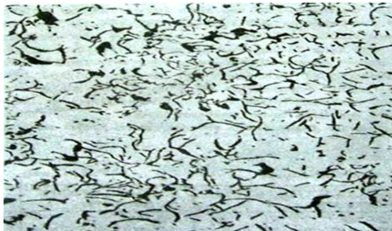
Fig.7.3 – Graphite flakes in gray cast iron
