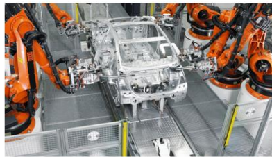
98% of the spot welding on Ford's Taurus by Robots
