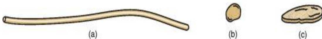
Fig.4.2 Possible physical shapes of imbedded phases in composite materials: (a) fiber, (b) particle (c) flake.
